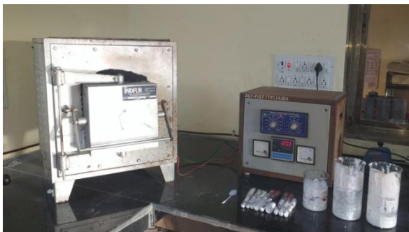
FIGURE 1. Sample being calcinated at 1200°C in a furnace
