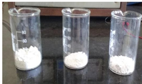
FIGURE 2. Samples after being calcinated at 200°C, 600°C and 1200°C
